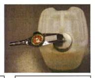
Step 4. Torque the cap to 150 in-lbs.
