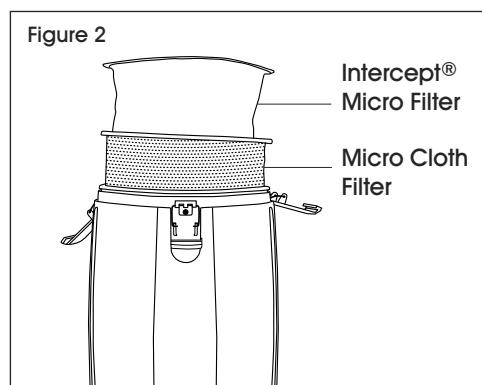
2. Replace if necessary. A clogged and dirty filter restricts airflow and results in reduced suction and overheating.
