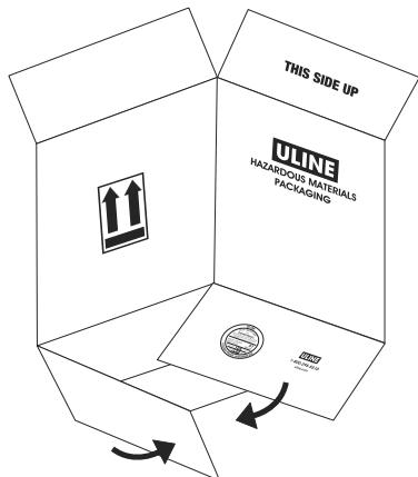
1. Fold flaps on bottom of carton so that they meet. Manufacturer's certification must be visible on the outside of the carton. (See Figure 1)
