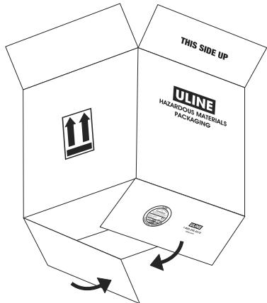
1. Fold flaps on bottom of carton so manufacturer's certification is visible on the outside of the carton. Gap between outside flaps cannot exceed 0.125". (See Figure 1)
