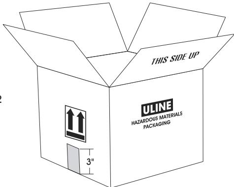
2. Seal bottom of carton down the center seam with one strip of 2" wide (2 mil) polypropylene tape (Uline Model # S-472). The tape must extend 3" over each end of the carton. (See Figure 2)
