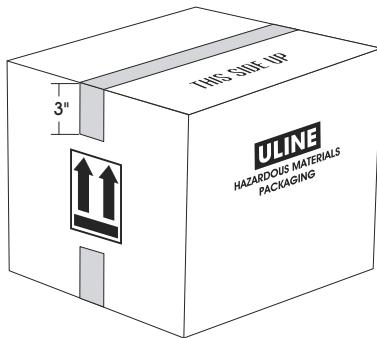
9. Seal top of carton down the center seam with one strip of 2" wide (2 mil) polypropylene tape (Uline Model # S-472). The tape must extend 3" over each end of the carton. (See Figure 6)
