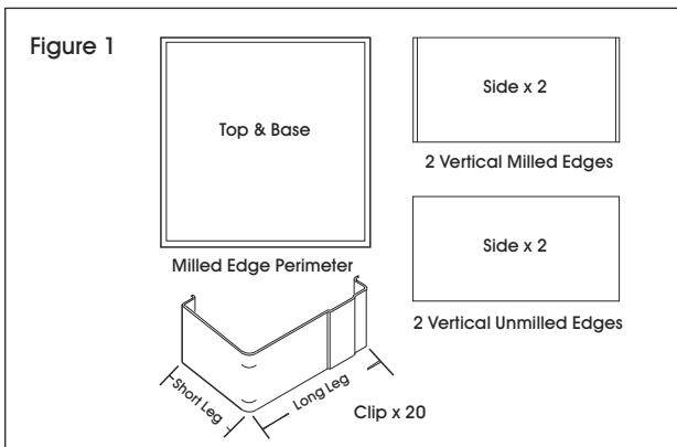
2. Attach milled-edge side to base with clips. (See Figure 2)
