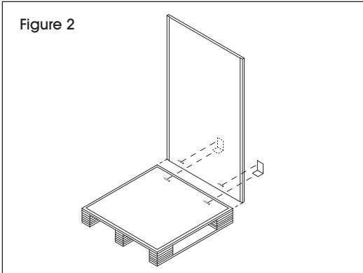
4. Attach unmilled-edge side to milled-edge side and base. (See Figure 4)
