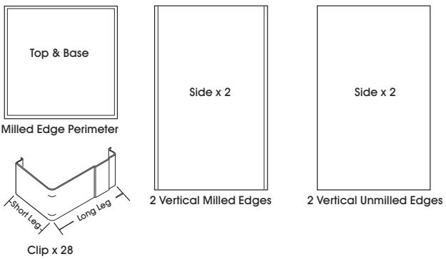
3. Attach clip so that the long leg spans across the edge of the overlapping board. Push the knee of the clip until it snaps into slot. (See Figure 3)
