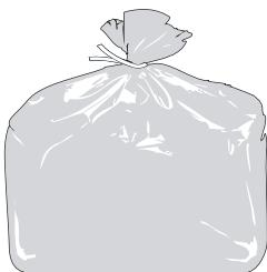
3. Place the air bag inside of the included 2 mil anti-static poly bag. Poly bag must be sealed with the included 5.5" 40# cable tie. (See Figure 3)
