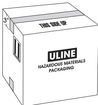
6. Fold flaps on top of carton so that they meet. "THIS SIDE UP" must be visible on the outside of the carton.
