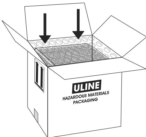
5. Place the bubble wrapped air bag into the center of the box. Fill any void space with 3/16" anti-static bubble (Uline Model # S-396). (See Figure 5)
