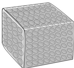
4. Wrap the air bag completely in 3/16" anti-static bubble (Uline Model # S-396). (See Figure 4)
