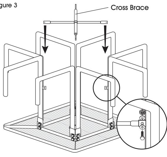
3. Align hole on cross brace between holes on table legs and attach using one bolt, two washers and one nut. Repeat for remaining three holes on cross brace. (See Figure 3)
