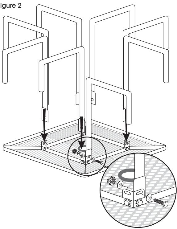
2. Attach legs to extension tab using one bolt, two washers and one nut. Repeat for remaining three extension tabs. (See Figure 2)
