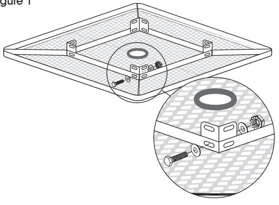
1. Flip tabletop so underside is facing up. Attach extension tab to square top using one bolt, two washers and one nut. Repeat for remaining three extension tabs. (See Figure 1)
