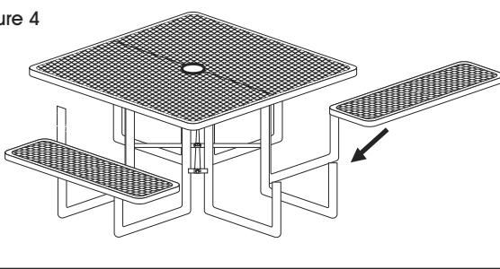
4. Flip the table upright. Attach seats to legs using one bolt, two washers and one nut. (See Figure 4)
