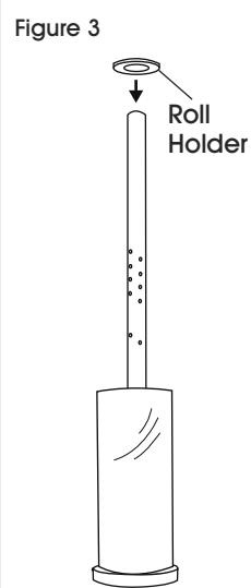
2. Insert 3" core stretch wrap roll over stem. (See Figure 2)
