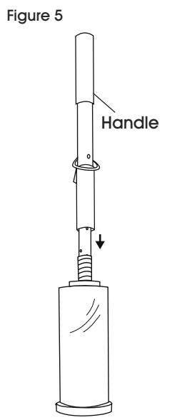
6. Adjust handle to desired tension by compressing spring and inserting tension control pin through desired holes.
