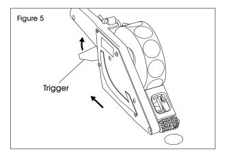
1. To apply label, squeeze trigger and pull machine toward user at a steady speed. (See Figure 5)
