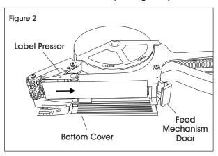
3. Push bottom cover closed. Lock feed mechanism door by snapping it into place. (See Figure 3)
