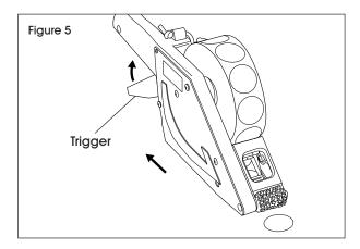
1. To apply label, squeeze trigger and pull machine toward user at a steady speed. (See Figure 5)
