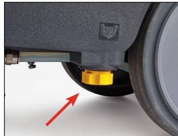
5. Clean the detergent drain filter by unscrewing the tank filter cap and removing the filter assembly. Clean thoroughly and re-secure in place. (See Figure 23)
