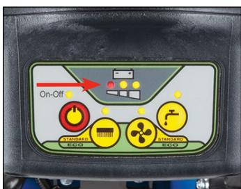
9. To recharge batteries, plug in battery charger using electrical cord provided with machine. Charge is complete when the green LED light is on. (See Figures 28 and 29)
