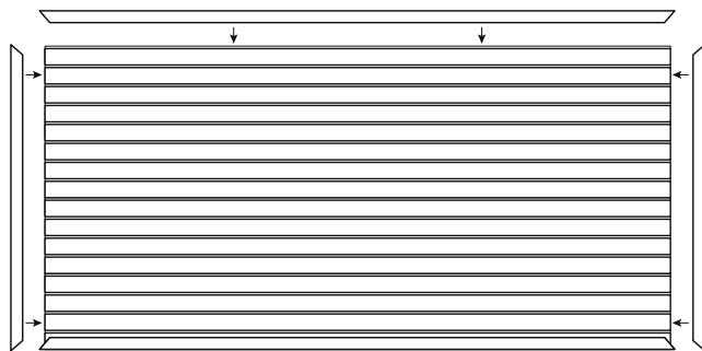
6. Slide three remaining miter cut J trim pieces into place. Adjust until corner pieces fit together. Tighten all screws to wall. (See Figure 6)
