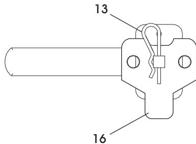
3. With the handle still in the open position, hook the lock bars (15) into the locking cam (16). Once in position, slowly rotate the door handle to the closed position so the lock bars protrude from the holes at the top and bottom of the door. (See Figure 11)
