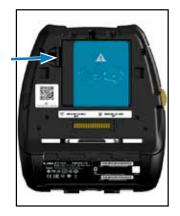
3. Rotate the pack away from the battery well. Lift the battery up and out of the printer.
