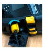
2. Rotate locking cap clockwise to secure.
