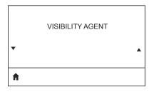
When the printer is connected to a wired or wireless network, it will attempt to connect to Zebra's Asset Visibility Service via the Cloud-based Zebra Printer Connector using an encrypted, certificate-authenticated web socket connection. The printer sends Discovery Data and Settings and Alerts Data. Data printed via any label formats is NOT transmitted. To opt out of this feature, disable this setting.
