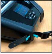
1. Insert the end of the shoulder strap behind the post on the front side of the printer and loop it around the post.
