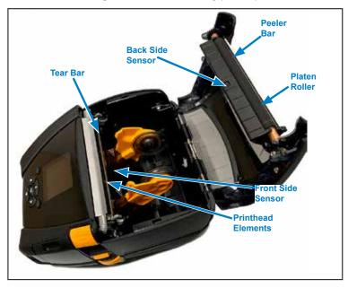
Figure 33 • ZQ630 Cleaning (Linerless)
