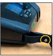
2. Insert the hole on the end of the strap over the metal post (circled) to secure.
