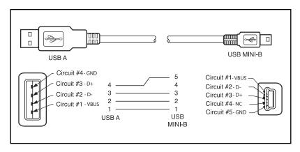
Part Number P1031365-055; 4 Position USB Mini to 4-Pin USB (w/ Strain Relief)
