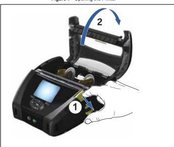
Figure 7 • Opening the Printer
