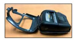
2. Rotate the top half of the Hard Case shell over the top of the printer and snap shut.
