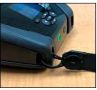
2. Loop the end of the strap back around the cut out and secure it over the button.
