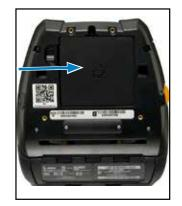
3. Insert the battery into the printer as shown. (It is not possible to insert the pack in the incorrect orientation.)
