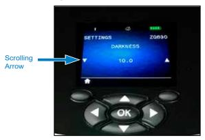
Some parameter settings like the Darkness setting above have a scroll option to view multiple setting choices. This option is identifiable by the presence of up and down scrolling arrows located on either side of the display (see Figure 14). Press the up and down arrows on the keypad to scroll through a menu's options. In some cases, further actions will appear on the right side of the status screen (see arrow in Figure 15). Press the right soft key to initiate said action.
