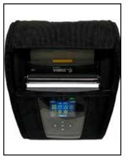
2. Slide the printer into the case such that the LCD display is visible through the plastic window.
