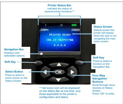
Figure 12 • LCD Control Panel
