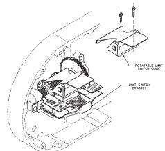
Figure 19A. Rotatable Limit Switches, Models J-RRT
