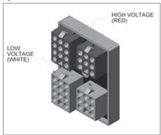
Figure 12. Voltage Change Board
