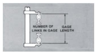
Figure 16. Gaging Load Chain Wear
