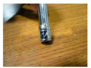
Tool Required: 1/4" Nut Driver with deep socket (Max. O.D. 3/8") note: a socket with a 3/8" drive will be too big and will not go into screw hole.
