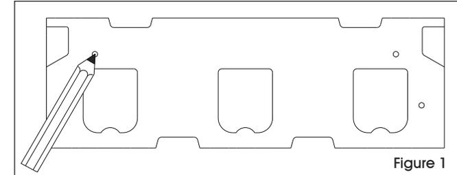
**NOTE:** Holes in the mounting template have 16" spacing to accommodate U.S. stud configuration.
