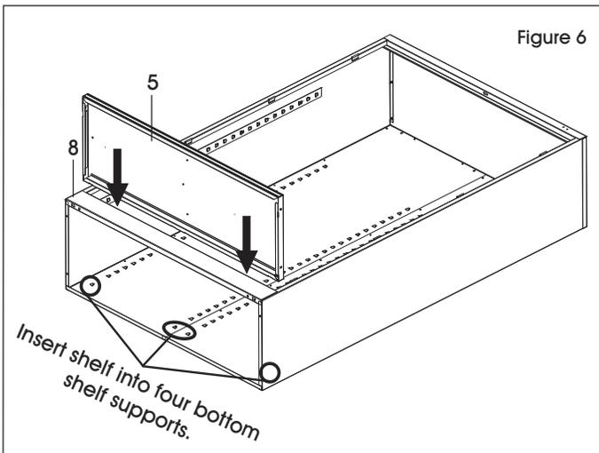
7. Using two people, set unit upright and tighten all nuts and bolts. Insert the remaining shelves. Be sure the shelf edge with no slots faces the cabinet front. The slots on the other three sides fit over the shelf supports on the cabinet walls, which hold the shelf in place.
