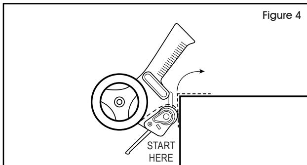
2. Pull the dispenser across the top of the box, applying pressure to the applicator roller to obtain a tight seal.
