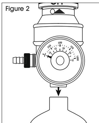
3. Connect the plastic bump test tube to the flow regulator outlet by sliding the tube over the grooves of the outlet.
