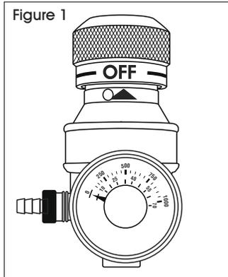
2. Screw the flow regulator into the calibration gas cylinder, making sure there is a tight seal. (See Figure 2)
