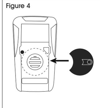
5. Make sure the detector is turned on before performing a bump test or calibration test.
