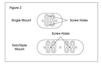
2. Screw the back plate to the wall using previously marked screw holes.
