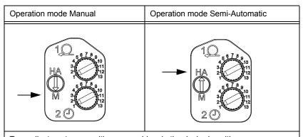
Turn adjustment screw with a screw driver in the desired position. Confirm the choice of the operation mode by pressing the tension button shortly.
