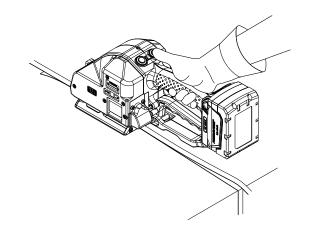
Release the tension button after the sealing process has been started.
