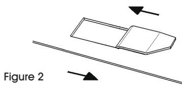
4. Tap the locking tabs down with a rubber mallet to tighten the connections.
