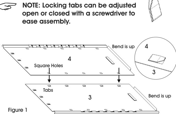
3. Once all the locking tabs are placed into square holes, slide the back panels in opposite directions to fully engage the tabs. (See Figure 2)
