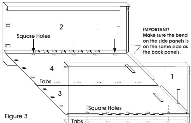
4. Tap each of the locking tabs down with a rubber mallet to tighten the connections.
