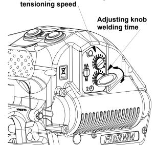
Adjusting knob tensioning force /
