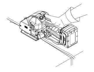
Release the tension button after the sealing process has been started.
