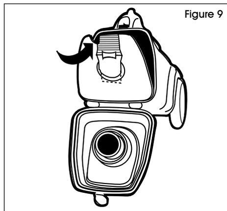
4. Check motor filter. If necessary, replace or clean by rinsing under warm water. Install when completely dry. (See Figure 10)
