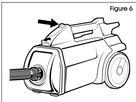
2. Press with hand or foot once to turn on. Press again to shut off.
