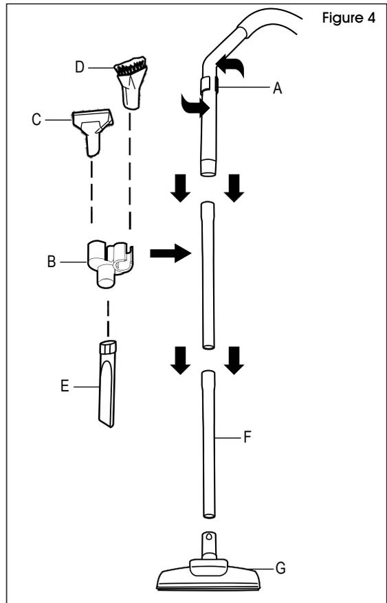
5. The telescopic wand (F) adjusts to different cleaning heights and the combination floor tool (G) works on both carpet and hard surfaces. (See Figure 4)
