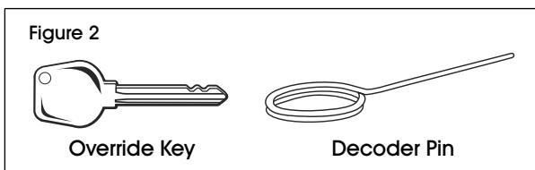
2. To use the override key, simply insert it into the keyway and turn the latch; the cabinet door will open and the lock may then be decoded. (See Figure 3)
