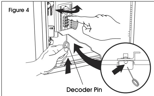
4. When you have located the correct number on the dial, the decoder pin will slip upward into an opening in the dial. The decoder pin will be fully inserted into the lock body when the correct numbers on all four dials have been reached. These four numbers are the lock's combination. You may then record the combination and keep it in a safe place or change the combination.
