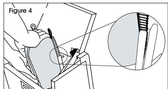
5. Once the cartridge is 3-4 inches below top of tracks, remove the yellow ribbon and cardboard. (See Figures 5-6)
