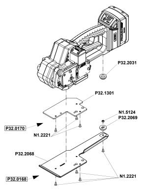
If the complete bottom side of the tool has to be protected, the plate P32.0168 must be used.
