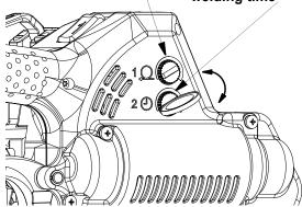
The adjustment knobs can be easily turned with a coin.
