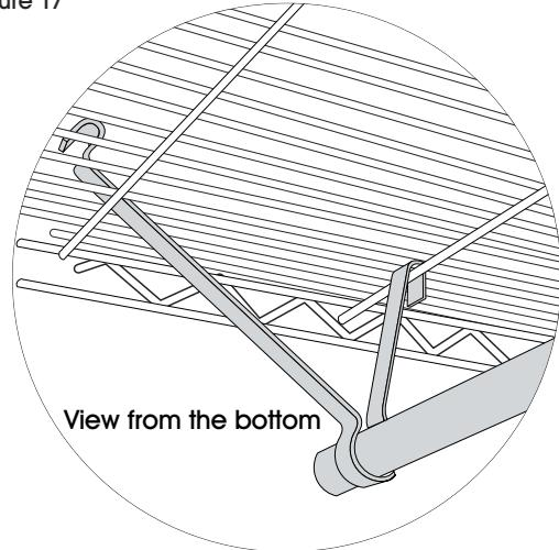
20. Pull garment rod back and down, one side at a time, until long end of garment rod hanger snaps into place.
