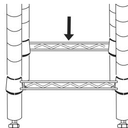
4. Position each of the four posts as shown and snap four sets of shelf supports into the groove directly above the square frames of the inner four posts. (See Figure 7)
