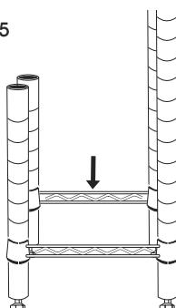
3. Take the other four tall posts, snap shelf supports into the very bottom groove on all four posts. Slide posts through underside of square frame until it slides firmly over the supports. (See Figure 6)
