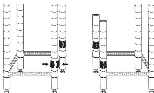
5. Slide a square shelf onto the inner four posts until it slides firmly over the supports. (See Figure 8)
