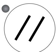
Push this RESET button, followed by the START button, to reset the system. The turntable will return to its home position and the carriage will lower.
