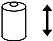
Turn the CARRIAGE SPEED adjustment knob clockwise to increase, and counterclockwise to decrease the carriage speed. This allows you to adjust the overlap of your film.
