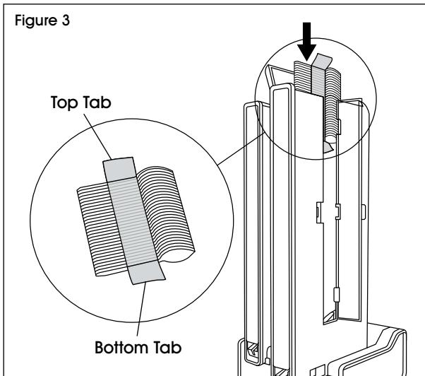
4. Remove tape by pulling top tab gently downward. Close top and side doors. (See Figure 4)
