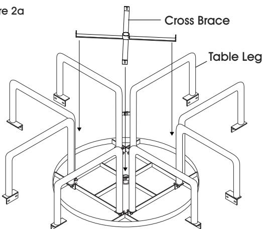
3. Insert the cross brace with the umbrella holder facing upward and loosely bolt to the corresponding corners using one bolt, two washers and one nut. (See Figures 2a-b)
