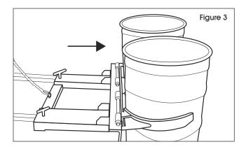
4. Lift the forks and the drum will be clamped and lifted. Carry the drum to the desired destination.
