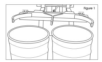
2. Slowly lower the forks to position the drum grabber clamps in the center of the drum. (See Figure 2)
