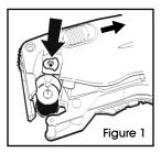
2. Hold the labeler sideways over a trash can while pushing the button to release the ink roller. (See Figure 1)
