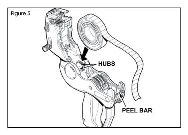
4. Place the label roll between the hubs and click into place. (See Figure 5)
