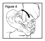
Pull the latches back and 1. swing the cover open completely. You should hear a click. (See Figure 4)
