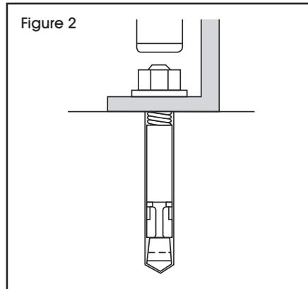
6. Tighten nut turning approximately three or four full turns.
