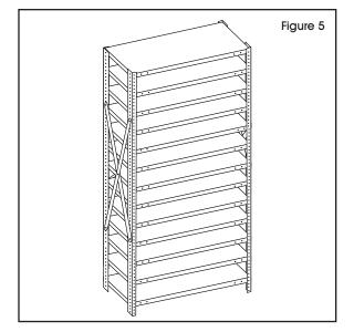
5. Stand unit up and tighten all bolts, use wrench. For 12" (H-1770) and 18" (H-1771) deep units, insert remaining shelves every sixth hole to evenly distribute. (See Figure 5)
