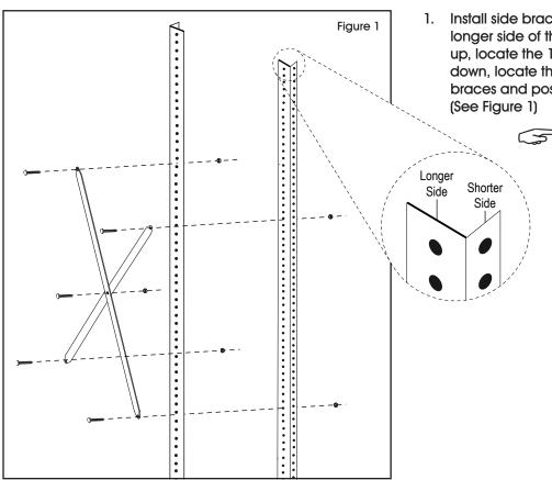
Install side braces: For 12" deep unit (H-1770), on the longer side of the posts, counting from the bottom up, locate the 19th hole and counting from the top down, locate the 24th hole. Insert bolts through side braces and posts. Tighten bolts with nuts. (See Figure 1)
