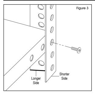
Install bottom shelf: For 12" (H-1770) and 18" (H-1771) deep units, align shelf with third hole up from bottom. Insert bolt through the shorter side of the post and through the shelf. Tighten bolts with nuts. (See Figure 3)
