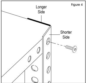
4. Install top shelf: For 12" (H-1770) and 18" (H-1771) deep units, align shelf with top hole. Insert bolts through the shorter side of the post and through the shelf. Tighten bolts with nuts. (See Figure 4)
