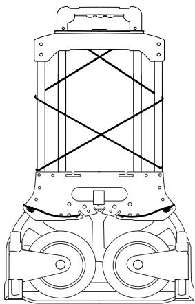
3. By pulling down the noseplate, both wheels will automatically extend out. (See Figure 3)
